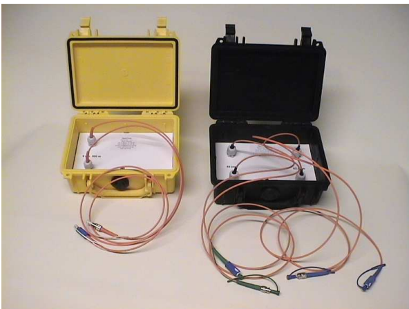
1 x 500m 9µm OS2, SC, FC/PC 2 x 100m 50µm + 62,5µm, ST, SC
